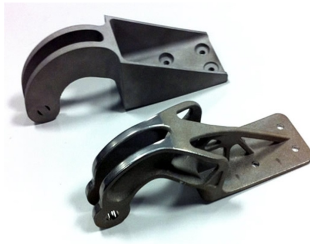
Figure 1: Traditionally manufactured latch on top. Latch re-engineered for AM at bottom. [5]
