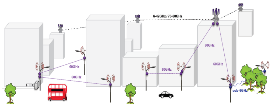
Figure 13: Small cell backhaul deployment possibilities.
