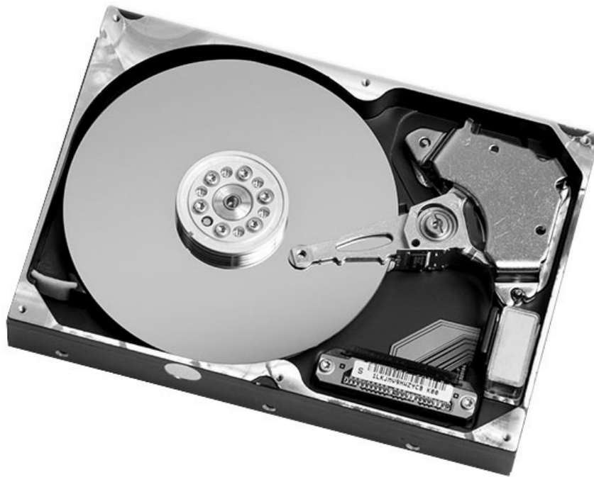
Figure 2.1: A magnetic disk's internal view. The currently inert disc that rotates rapidly while in use can be seen, as well as the read/write-head. Image credit: Flickr user Jeff Geerling, http://www.flickr.com/photos/lifeisapraye/2282011834 . Used with Creative Commons license: https://creativecommons.org/licenses/by-nc-sa/2.0/
