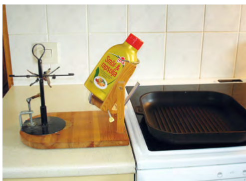
Figure 37. A tilting wooden stand for an oil bottle next to a stove.
