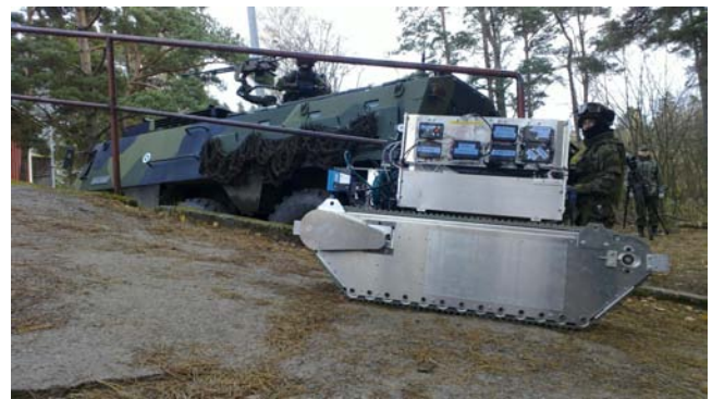
FIGURE 9. The mobile robot unit used for exploring, mapping and node localization in the MUSAS.
