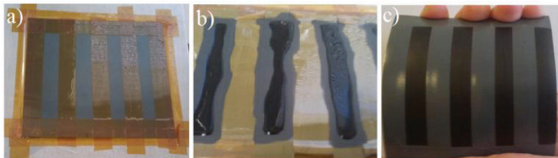
Figure (14 a-c): Demonstration of ink deposition a) patterning of the substrate, b) application of ink and evaporation of solvent at 120 °C in 5 minutes c) SWCNT patterns (Copyright Wiley-VCH Verlag GmbH & Co. KGaA. Reproduced from Publication 5 with permission).
