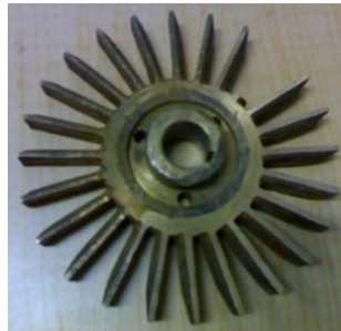
Figure 5 Broken impeller (one vane missing) (see online version for colours)
