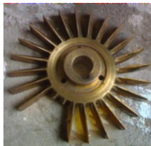
Figure 6 Broken impeller (two vane missing) (see online version for colours)
