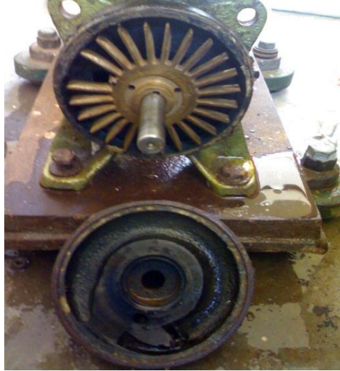
Figure 8 Broken impeller inside casing of the centrifugal pump (see online version for colours)
