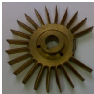
Figure 7 Broken impeller (three vane missing) (see online version for colours)
