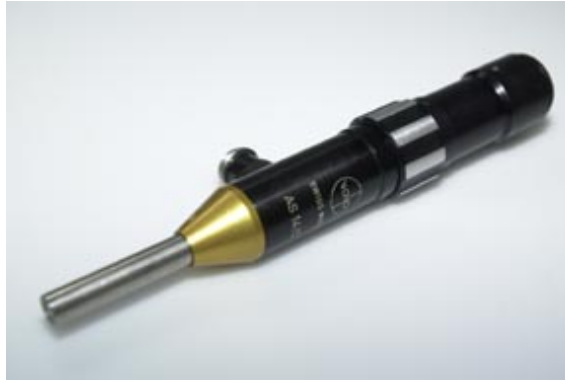
Figure 4.3. Volpi AS11/50 video microscope probe. A C-threaded mount for the camera is at the right. The long narrow tube extruding to the left houses the front lens element. The front lens is surrounded with optical fibers for coaxial illumination. The perpendicular illumination port for interfacing with a light source is at the back. Focusing is carried out with knurled focuser ring in the middle.
