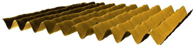
Figure 4: An example of surface-relief grating topology inscribed on an azobenzene-containing polymer thin film.
