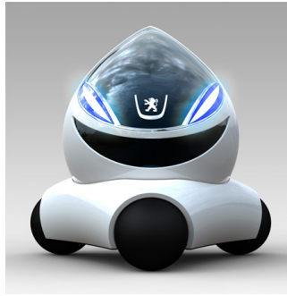
Figure 2.6: Ball wheels implemented on MoVille car concept. (Source: Woo-Ram Lee (2013))
