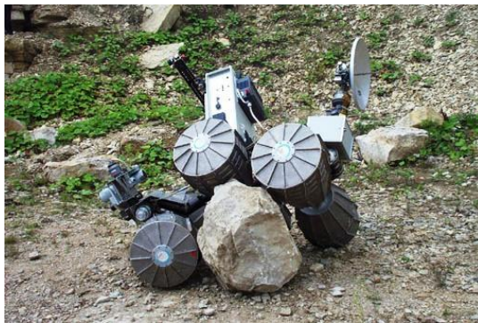
Figure 2.8: The articulated suspension of the Marsokhod rover. It is fully articulated in pitch, roll and yaw. (Source: Jean-Marc Maclou (2011))
