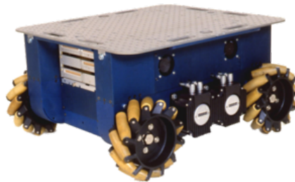
Figure 2.5: Mecanum wheels implemented on URANUS omni-directional mobile robot. (Source: Carnegie Mellon University (2011))
