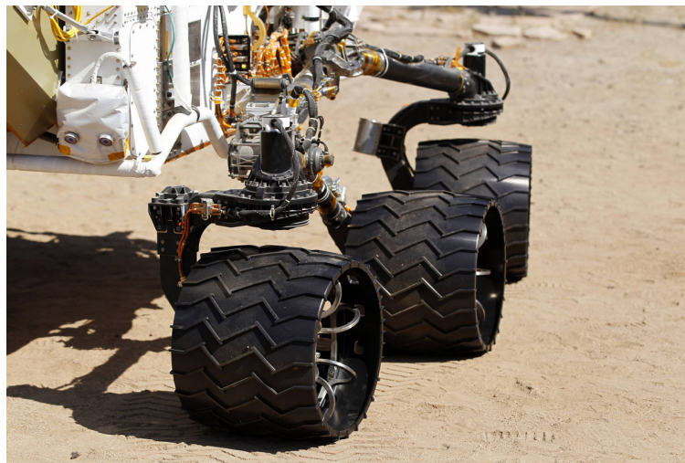
Figure 3.1: Three of six 20 inch aluminum wheels on an engineering model of the MSL rover. Steering axes are crossing the centers of the wheels. (Source: Tann (2012))
