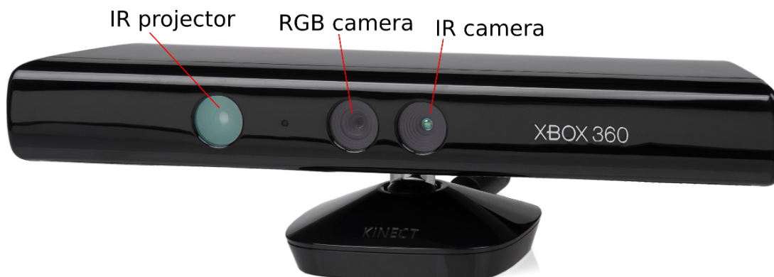
Figure 8: Kinect sensor with cameras and projector annotated. Picture adapted from [77]
