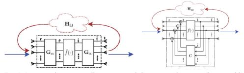
Fig. 5. Loop interference cancellation in spatial domain or subtraction of estimated loop interference.
