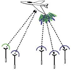
Fig. 8. Multistatic, MIMO Radar configuration using waveform diversity. Virtual aperture may be created using signal processing for designing and optimizing the waveforms launched from each antenna.
