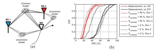
Fig. 2. (a) A multi-link GSCM based on the concept of common cluster (CC). (b) Sum rate capacity (SRC) comparison between measurements and simulations.
