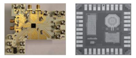
Fig. 14. a) Implemented wideband receiver b) Chip photograph of implemented synthesizer.
