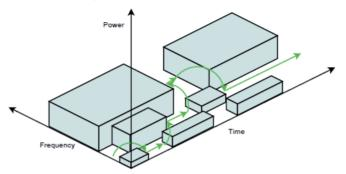
Fig. 12. Flexible use of time-frequency-location varying underutilized spectrum.
