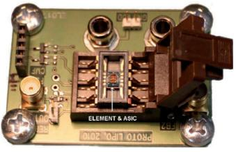
*Fig. 33. The prototype PCB, which also shows the sensor element and the ASIC, which are directly wirebonded.*
