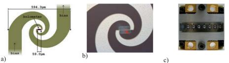
Fig. 27. a) Dimensions of microbolometer, b) a micrograph of the same, c) a module of eight bolometers with silicon lenses.
