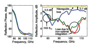
Fig. 20. Measured  $S_{11}$ -parameter of the reflection type phase shifter with MEMS tunable HIS over W-band. Reflection phase is 0° at the resonance frequency of 83.4 GHz. Minimum insertion loss of the HIS outside of the resonance is 0.7 dB.
