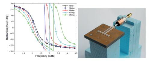
*Fig. 11. Reflection-phase diagram for an infinite HIS with two resonance bands (left). Manufactured and measured dual-mode antenna (right).*
