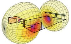
Fig. 1. Novel antenna structure with a capacitive coupling element (CCE, right) and a bowtie antenna (left). The unbalanced (CCE) and balanced (bow-tie) antenna elements have almost orthogonal radiation patterns.
