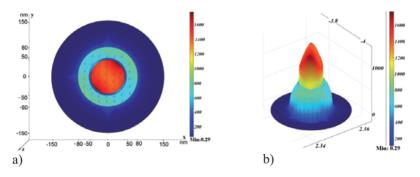
Fig. 29. Cross-section of the annular waveguide (a) and power flow distribution (b).
