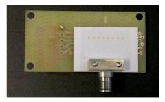
*Fig. 24. A photograph of the designed Rexolite lens with optimised eccentricity. A photograph of the feed array with eight aperture coupled patch antennas on LTCC.*
