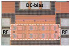
Fig. 17. Chip micrograph of the 94-GHz CMOS power amplifier. The area, including pads is 0.24 mm<sup>2</sup> (610  $\mu$ m x 400  $\mu$ m) and the active area (encircled with the dashed white line) is 0.069 mm<sup>2</sup> only.
