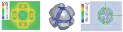
Fig. 34. (left) - Spatial distribution of the amplitude of electric field at 369 THz for an effective plasmonic loop comprising four dimers; (center) - A cluster made of eight triangular nanoprisms on a dielectric core; (right) - Spatial distribution of the electric field vector at 400 THz for the cluster comprising eight triangular nanoprisms.
