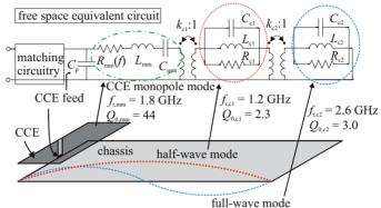
Fig. 15. Capacitive coupling element (CCE) on a ground plane (chassis) and the equivalent circuit model representing the CCE and the illustrated first two wavemodes that are excited on the ground plane.
