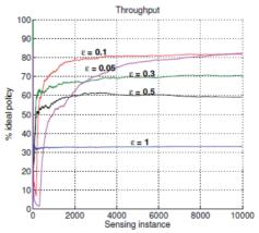
Fig. 13. Trading off between spectrum exploration and exploitation. Developed greedy spectrum sensing policy allocates sensing to subbands that provide idle spectrum persistently and as a result performance close to ideal sensing policy is achieved.
