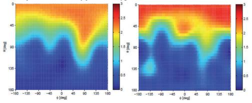
*Fig. 10. Simulated (left) and measured (right) directivity patterns of a linearly polarized Huygens source comprised of two omega-particles.*
