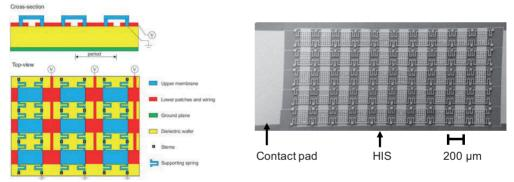
*Fig. 19. Multilayer MEMS tuneable high-impedance surface (part of a larger array shown): design (lhs) and SEM image of the fabricated prototype (rhs).*
