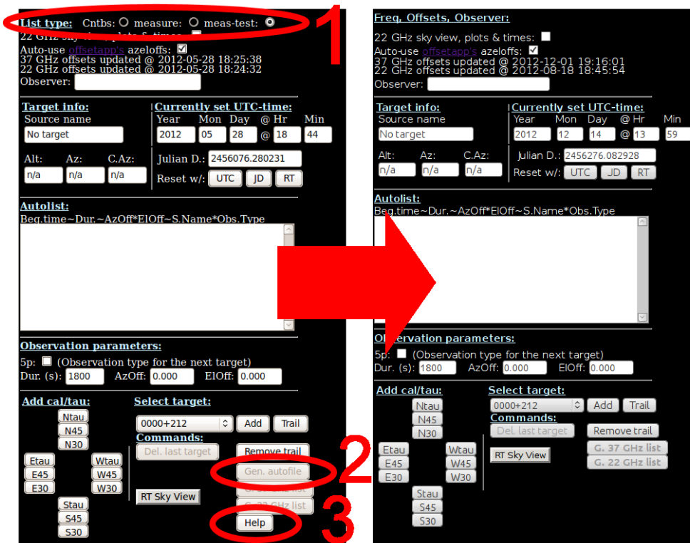
Figure 28. The changes made to the autofile generator based on the heuristic evaluation of the first evaluation round. On the left is the user interface as it was in 2012-05-28 and on the right the version in use in 2012-12-14. The removed controls are highlighted with red ellipses and numbered from 1 to 3. 1. The list type selectors were hidden because currently only one list type is in use. 2. The Gen. Autofile button was hidden because the list type it creates is no longer in use. The Help button was hidden because no actual help was available by pressing it.
