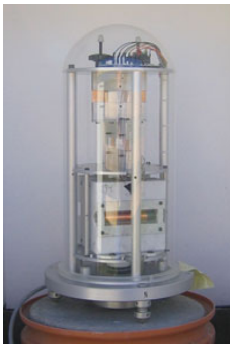
Figure 5: Danish FGM-FGE fluxgate magnetometer, one of the most widely used observatory magnetometers in the world.[49]
