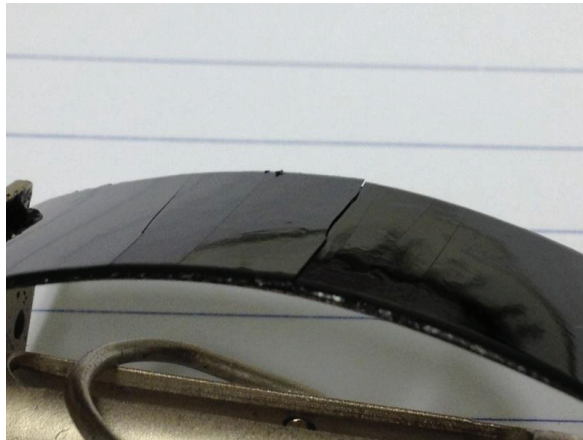
Figure 21. Binder film cracking on Fraass breaking point measurement test: example of large crack easy to see and smaller cracks more difficult to detect by naked eye during testing.
