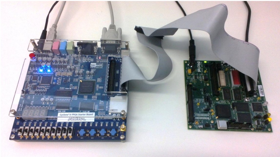
Figure 27: The Cyclone (left) and IGLOO FPGA development kits connected together, powered up, and running the PLS
