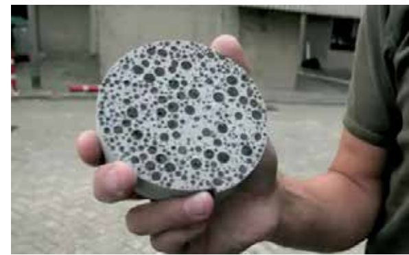
Picture 161. Self-healing BioConcrete that contains bacteria. When concrete cracks, bacteria will heal the crack decreasing need for maintenance.
