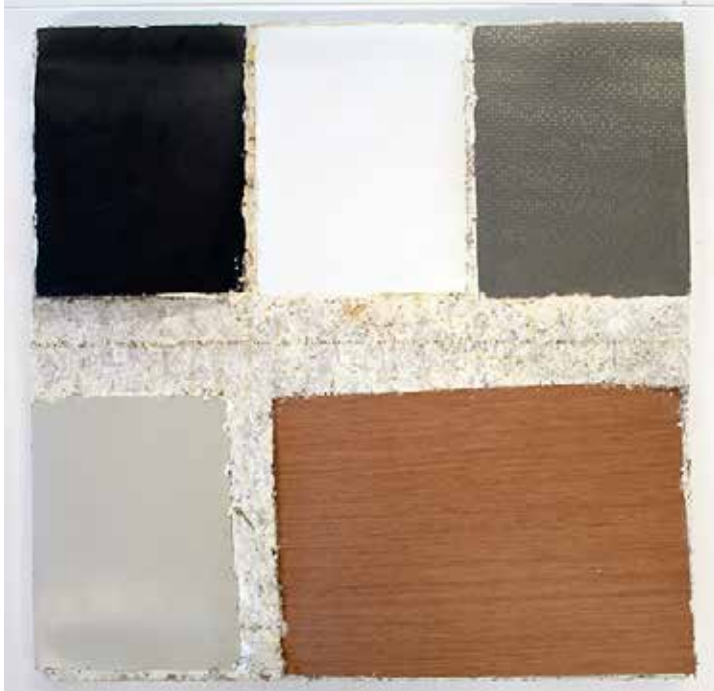
Picture 166. One of the test samples where mycelium was grown on lamination. More stiff the lamination, the better result.
