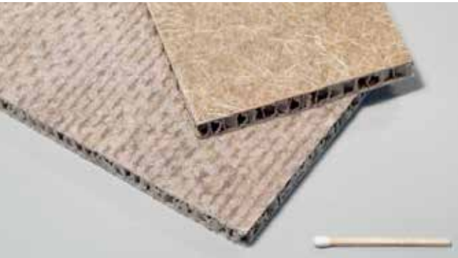
Picture 151. Duroplastic has cardboard honeycomb core.
