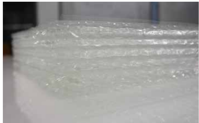
Picture 44. Moniflex, an insulation panel made of cellulose, was used already 60 years ago in trains (Peters 2011, 38).
