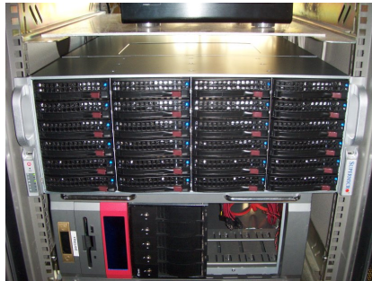
Figure 1.6. The fully-COTS 4U 36 disk chassis platform (Supermicro SC847A-R1400B).
