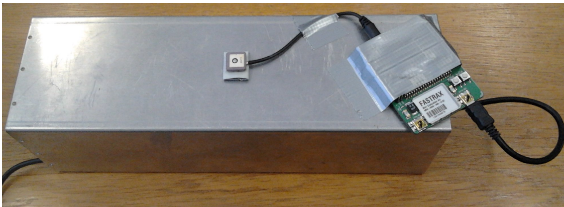
Figure 27: An Adactus ADA-15S antenna attached to an mockup aluminium frame was used in antenna performance testing with a Fastrax Mini Evaluation Kit.
