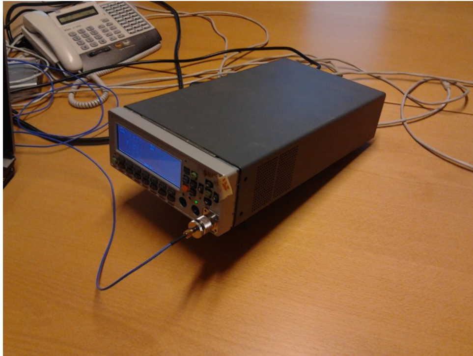
Figure 20: A modified Spectracom GSG-55 GPS signal simulator.
