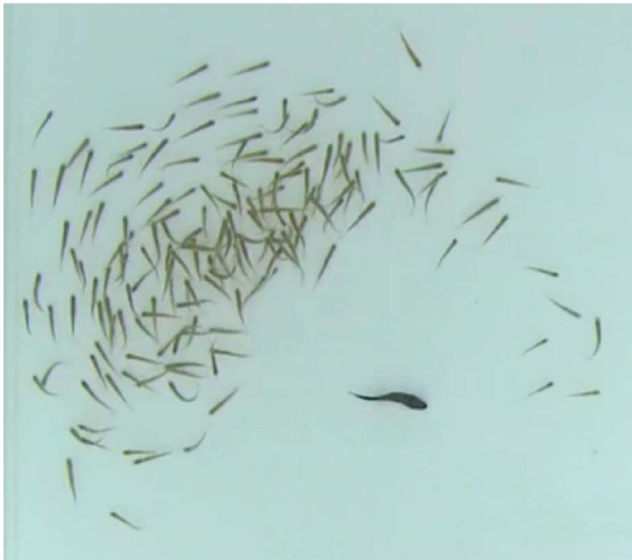
Figure 1.2: Overhead snapshot of robotic koi predator with live golden shiner school in a tank [6].
