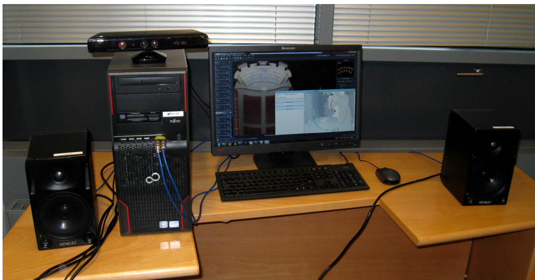
Figure 1.1: An example setup, including a set of speakers, a Microsoft Kinect, and a PC running Conductor Follower along with a synthesis environment, Vienna Ensemble [19].
