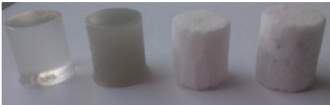
Figure 36. Samples for compression testing. From right: PCL, PCL-BAG, p-PCL and p-PCL-BAG-titanium.
