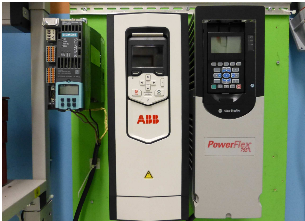
Figure 16: The three AC drives mounted on the wall, in order from left to right (with dimensions height x width x depth in mm): SINAMICS S110 (195 x 73 x 216) by Siemens AG [2011c], ACS880-01 (405 x 155 x 226) by ABB [2012d], and PowerFlex 755 (424 x 134 x 212) by Rockwell Automation, Inc. [2011]. Only supply cables are wired to the drives.
