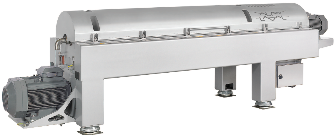
Figure 6: The Alfa Laval [2006] decanter model P2-405 for process industries, with maximum dimensions of 457 x 111 x 160 cm (length x width x height) and a weight of 3,800 kg. The bowl, hidden inside, has a diameter of 450 mm and rotates at the maximum speed of 3250 rpm. The inlet is visible at the left side, above the main motor. The back motor is partly visible at the other end of the decanter. Outlets for solids and liquids are hidden in the bottom, between the stands. (Figure courtesy of Alfa Laval Corporate AB [2012] press material.)
