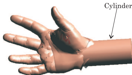
Fig. 4.5. Hand and wrist model used in the wrist mode. The size of the hand corresponds to that of an average human hand, but the length of the cylindrical wrist is only indicative.
