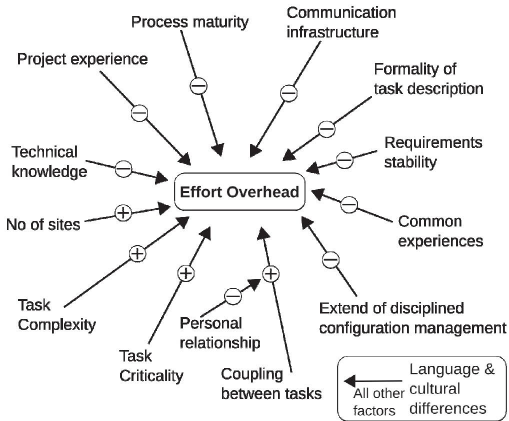
Figure 21: Causal model for cost estimation of global software development (Lamersdorf et al., 2010)
