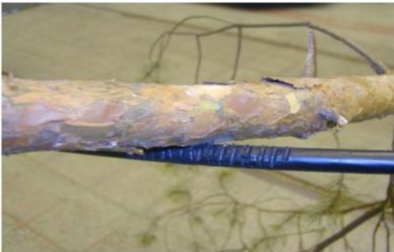
Fig. 3.4 Knife traces are made and a pine tree is leaned on the conductor insulation [3].
