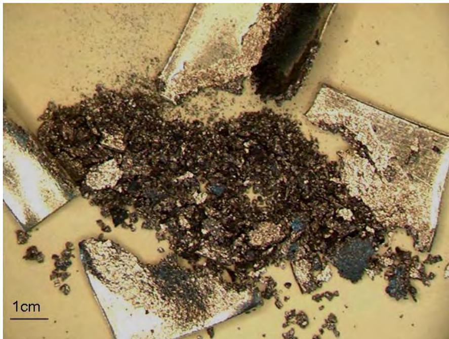
Fig. 3-12 Sn pest in pure Sn plate after 50 hours at  $-196^\circ\text{C}$  plus 4 years at  $-40^\circ\text{C}$  and plus 1.5 years at  $-17^\circ\text{C}$ .
