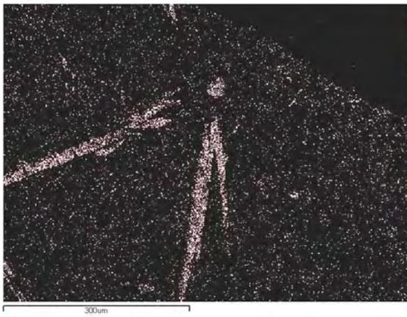
Fig. 4-3a Cu mapping revealed the primary phase  $\text{Cu}_6\text{Sn}_5$  in Ames alloy (Sn-4.7Ag-1.7Cu).
