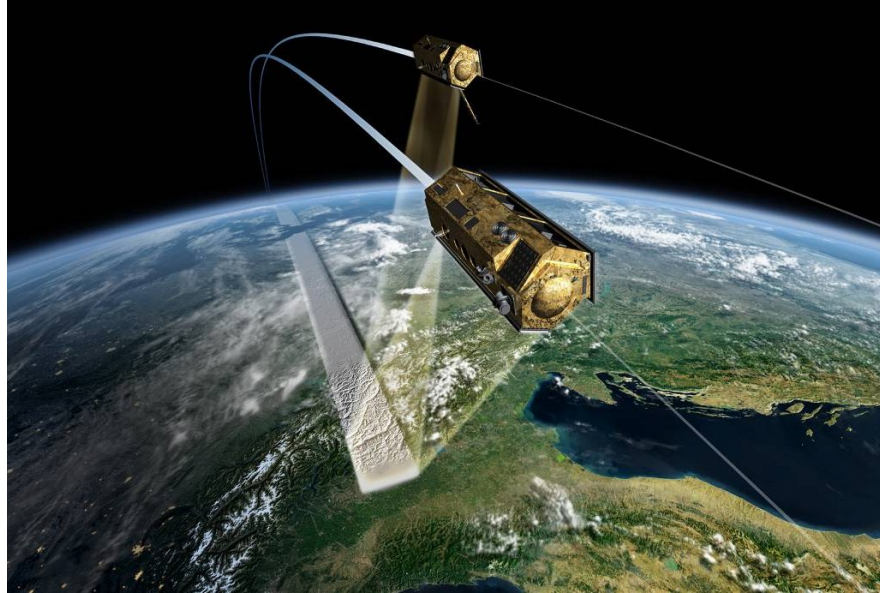
Figure 3.2: TanDEM-X and TerraSAR-X flying in formation. Image from (15).
