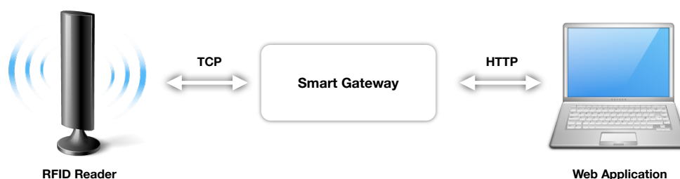
Figure 2.5: A Smart Gateway as mediator between an RFID reader communicating with TCP protocol and a Web application.
