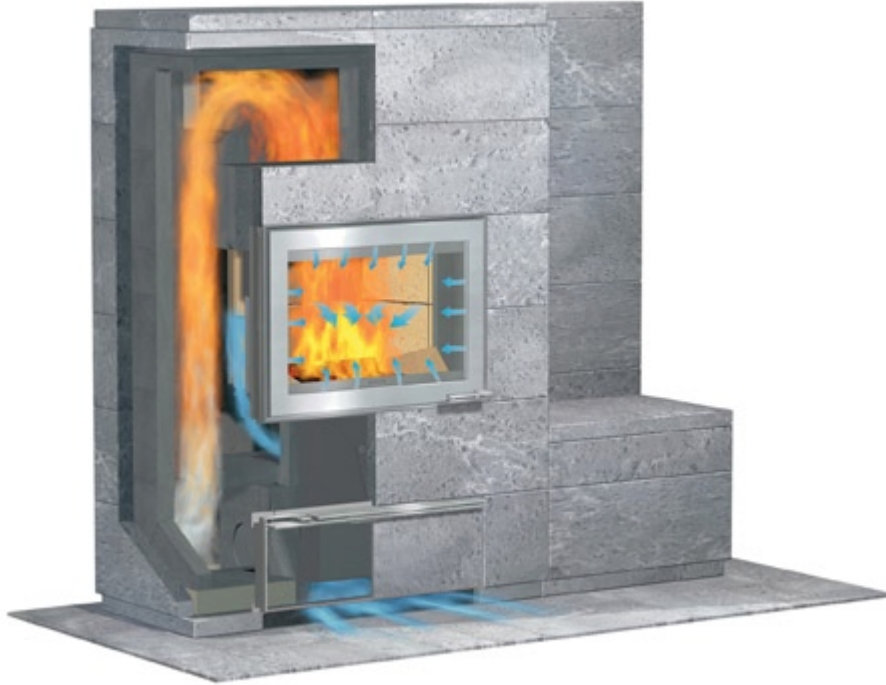
Figure 2.3: A modern masonry heater. The arrows indicate the intake air. (Alakangas et al., 2008b)
