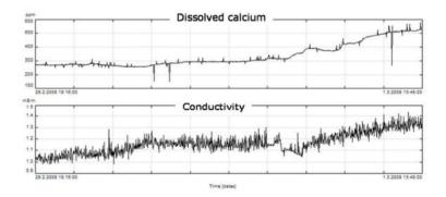
**Figure 24** Conductivity (with YSI 6920V2) and the amount of dissolved calcium (with Consort C933 equipped with online sample pretreatment) measured in the wire pit. *Paper III*.
