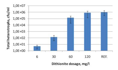
**Figure 40** Effect of dithionite on the biocidal efficiency against aerobic bacteria of electrochemically generated hypochlorite in a clear filtrate from a board machine. Biocide dose was 44ppm as free active chlorine. REF = Clear filtrate without biocide treatment. Error bars represent standard deviation between three independent experiments. *Paper I*.
