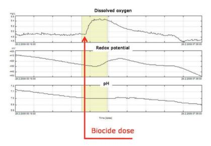
**Figure 29** The effect of oxidative biocide feed on dissolved oxygen, redox potential, and pH measurements (measured with YSI 6920V2). A coloring presents the dosing batch of the biocide. *Paper III*.
