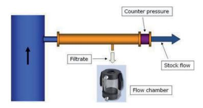
Figure 10 Ceramic filter connected to a flow chamber for filtrate.
