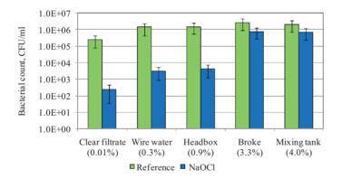
**Figure 37** Biocidal efficiency of electrochemically formed hypochlorite against bacteria in samples from different process stages of fine papermaking. The consistency of the sample is presented below the name of the sample. Hypochlorite addition was 3ppm. Error bars represent standard deviation between three independent experiments. References indicate the samples without biocide addition. *Paper II*.
