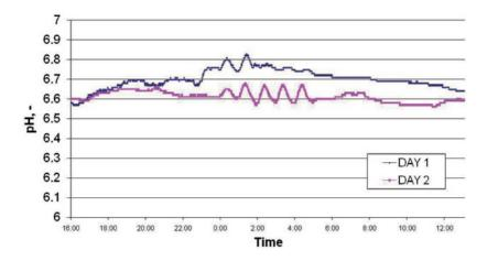
**Figure 26** pH in the water removal chest during felt washing measured with YSI 556MPS. *Paper III.*
