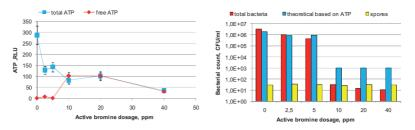
**Figure 22** Optimization of biocide dosage with a portable ATP luminometer. Biocide was dosed to fine paper machine's clear filtrate. Viable bacteria were calculated on the basis of intracellular ATP, which was estimated by subtraction of free ATP from total ATP content. ATP values are averages of at least three measurements. *Paper IV*.
