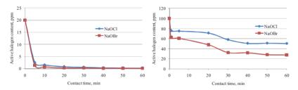
**Figure 43** The decomposition of electrochemically formed hypochlorite and hypobromite in a bacteria free clear filtrate when the initial biocide concentration was 20ppm (left) and 100ppm (right). *Paper II*.
