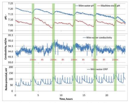
Figure 28 Chemical variations in the short circulation due to the biocide addition. Colorings present the batch-wise added biocide dosing. *Paper V*.
