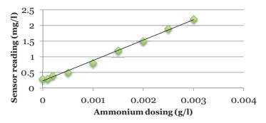
Figure 18 Response of ISE ammonium measurement (YSI Professional Plus) to ammonium dosing into process water sampled from a paper machine.
