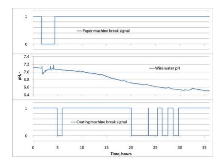
Figure 33 The effect of PM break on chemical stability of the PM wet end and PCM runnability. *Paper V*.
