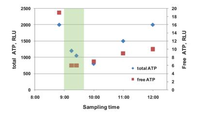
**Figure 17** ATP (free and total) measurements on wire water to monitor the effect of biocide performance. Coloring presents the dosing of biocide (hypochlorite was added for 40 minutes time). *Paper IV*.
