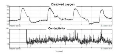
Figure 21 The effect of biocide feed on dissolved oxygen and conductivity measurements. Both parameters were measured with YSI 6920V2. *Paper III*.
