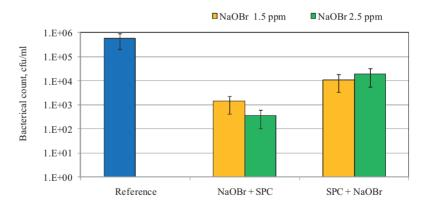
**Figure 42** Effect of dosing order of electrochemically formed SPC and hypobromite. Sample treated was the clear filtrate from a fine papermaking. Hypobromite addition was 1.5 and 2.5ppm. SPC addition was 50ppm. Error bars represent deviation between 3 parallel platings. Reference indicates the sample without biocide addition. *Paper II*.
