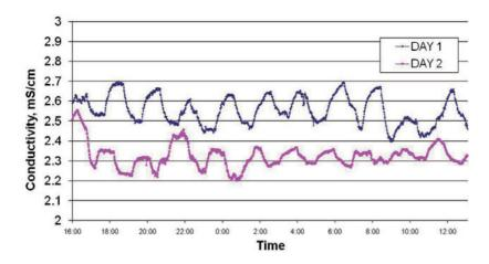
**Figure 27** Periodical fluctuations in water removal chest conductivity (measured with YSI 556MPS). Same time period and measurement location is presented as in the Figure 26. *Paper III*.
