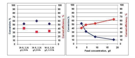
**Figure 34** Conversion and current efficiency at different operating conditions (left) and the effect of NaCl feed concentration on conversion and current efficiency (right), current 20A and flow rate 8l/h.
