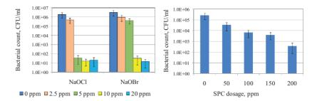
**Figure 35** Efficiency of electrochemically formed biocides in fine papermaking clear filtrate. The dosage is presented as active substance (free active chlorine, free active bromine, or hydrogen peroxide). Error bars represent standard deviation between three independent experiments. *Paper II*.
