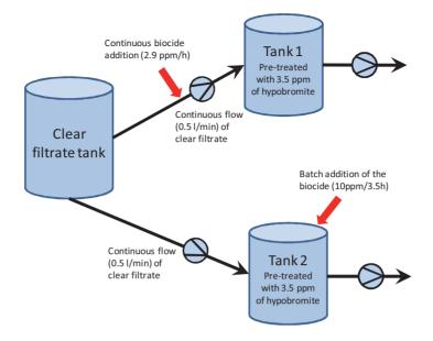
**Figure 12** Trial setup for the determination of the effect of dosing mode. Flow rates of the pumps were synchronized so that the clear filtrate levels in the tanks 1 and 2 were constant.
