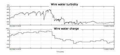
**Figure 23** Online turbidity (measured with YSI 6920V2) and charge (with Mütek PCT20) measured from a flow after the wire pit. *Paper III*.
