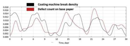
**Figure 32** Correlation between base paper defects and coating machine runnability. Break density and defect count are calculated according to equations 1 and 2. *Paper V*.
