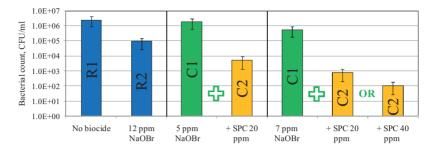
**Figure 41** Combined effect of electrochemically formed hypobromite (C1) and SPC (C2) in broke. C2 bars (orange color) present the combined effect of hypobromite and SPC. R1 and R2 present the reference trials; C1 is component 1, and C2 is component 2. Error bars represent deviation between 3 parallel platings. *Paper II*.
