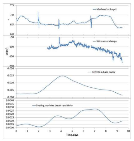
**Figure 15** Observed chemical variations at a paper machine and their influence on paper defects and runnability in coating. Break sensitivity and defects curves are calculated according to equations 1 and 2. Modified from *Paper V*.
