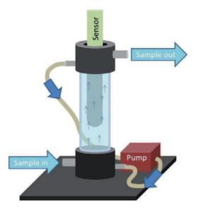
Figure 11 Flow chamber with auto-stirring system.
