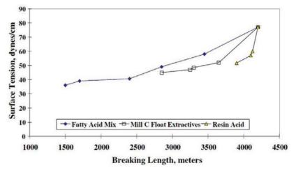
Figure 4 Relationship between surface tension and breaking length as a function of contaminant additions (Tay 2001).
