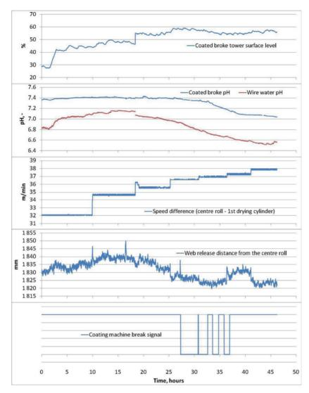
**Figure 16** Effect of broke spoilage on web adhesion and coating machine runnability. *Paper V*.
