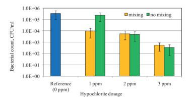
**Figure 38** Effect of mixing on the clear filtrate biocide treatment efficiency with electrochemically formed hypochlorite. Error bars represent deviation between 3 parallel platings. Mixing was applied with a three-blade mixer with rotation speed 180rpm. *Paper II*.
