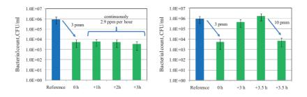
**Figure 39** Comparison of continuous (left) and batchwise (right) addition of biocide to the clear filtrate. Electrochemically formed hypobromite was used as the biocide. Error bars represent deviation between 3 parallel platings. Reference indicates the sample without biocide addition. *Paper II*.
