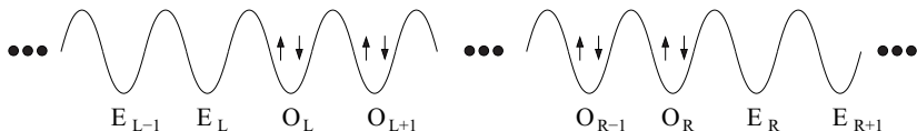
Figure 3.4. Schematic representation of the initial state: the middle part of the lattice is fully occupied ( O_i ) and the rest is empty ( E_i ). Sites E_L , O_L and O_R , E_R represent the left and right edge of the cloud, respectively.
