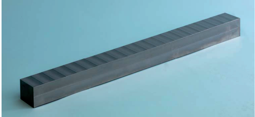
Figure 27 The calibration block consists of 22 thickness steps ranging from 38.9 mm to 41.0 mm.
