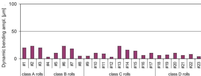
Figure 76 Dynamic bending of backing rolls at a web speed of 1400 m/min. The rolls are grouped by generations.
