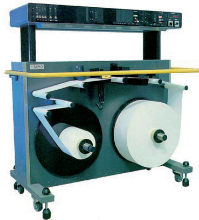
Figure 39 Tapio PMA is used for analysis of both machine and cross direction samples of paper. (Fig: Tapio PMA for CD Applications. Tapio Technologies Oy).
