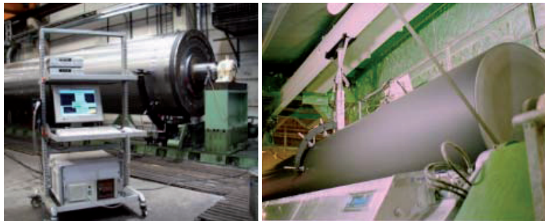
Figure 42 Measurement setup at a roll workshop (left) and at a coating station of a paper machine.
