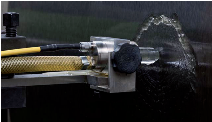
Figure 26 The thickness map of a rotating roll is measured using a ultrasonic squirter probe in which the cutting fluid transmits the sound waves from the transducer to the measured object.
