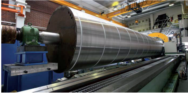
Figure 21 The test roll at the laboratory grinding machine. White painted stripes were used in testing for better surface quality in the laboratory measurements to test a possible improvement in a performance of laser sensors.
