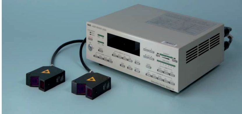
Figure 17 The 2-channel laser displacement sensor unit Matsushita Nais LM300/R30 uses diffusive reflective triangular laser beam technology.
