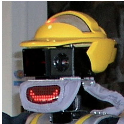
Figure 5.1.2: Close-up photograph of WorkPartner's head equipped with laser pointer and color camera.
