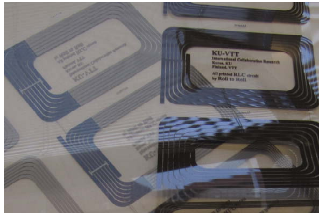
Figure 22. Wireless RF resonant tags R2R gravure printed using silver nanoparticle and dielectric inks 7 .
