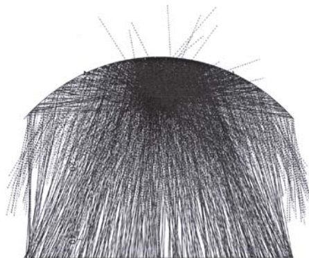
Fig. 3.18 Ray tracing of flashing energy in the experimental set-up.
