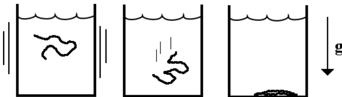
Figure 1.2: A cartoon depicting polymer sedimentation. Left: A solvent including an added polymer is shaken. Center: The gravity \mathbf{g} acting upon the polymer makes it sedimentate towards to bottom. The different parts of the polymer interact via the complex fluid field that they exhibit. Right: The sedimentation process is ended as the polymer reaches the bottom.
