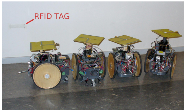
Figure 5.1: The MarsuBot robots (Danny, Emma, Fiona and Hugo) used in the laboratory experiments. An RFID tag serving as a landmark is visible in the background.
