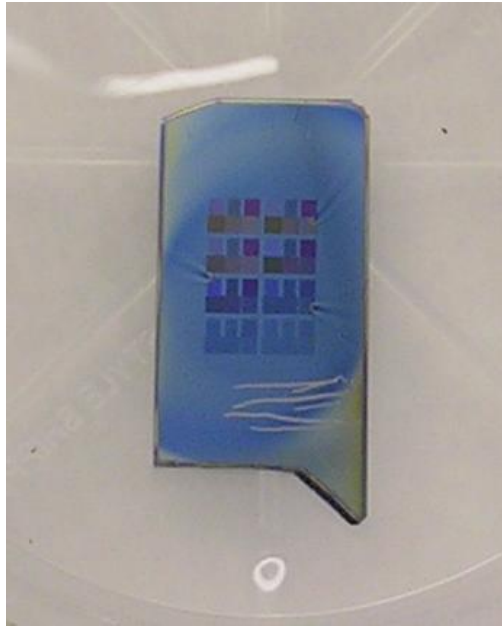
Figure 11.11. Test sample for electron beam lithography.
