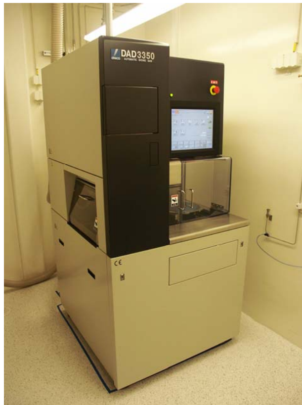
Figure 11.15. Dicing saw (Disco DAD3350).
