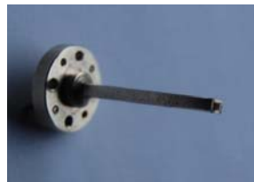
Figure 6.4. Open-ended WR-10 waveguide as a measuring probe.
