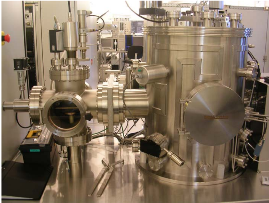
Figure 11.8. Evaporator for ohmic contact deposition.
