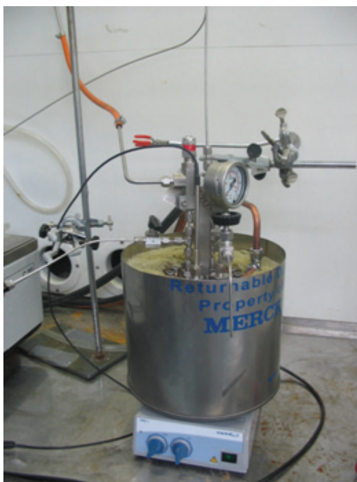
Figure 17. Photo of the test facility used for experiments performed at elevated pressures (Eloneva, 2008).
