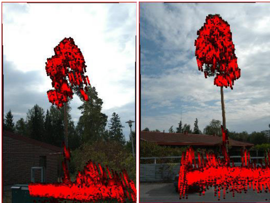
Figure 17. The full-waveform superimposed onto images. The difference in the viewing angles of the images is close to 90 degrees.
