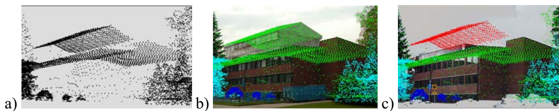
Figure 13. a) Perspective view of the ALS point cloud b) ALS data is integrated with the terrestrial image c) after half a year, the temporary structure was removed from the roof. (from Paper I)
