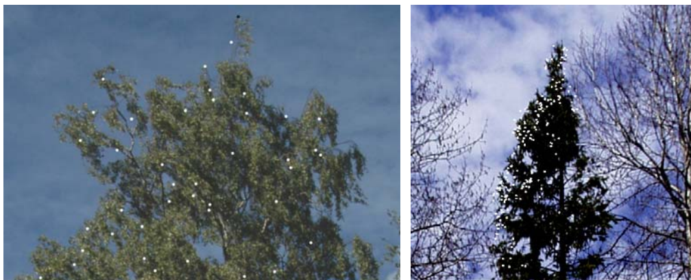
Figure 11. Leaf-on laser scanning has not found the highest top of the birch (left). The black spot indicates the actual treetop and the white ones represent laser data. The perspective causes a misunderstanding of the heights, because the treetop is observed from a worm's-eye view. The distance between the highest laser point and the actual treetop is 1.37 meters. Spruce is measured with about 50 pulses per square meter (right). Part of the spruce is shadowed by surrounding aspens. (from Paper IV)
