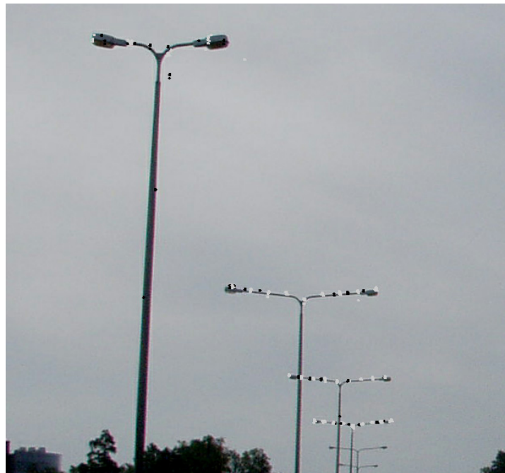
Figure 21. Integration of laser point clouds and a terrestrial image illustrates how the point density of both Toposys and TopEye has been sufficient to detect the upper parts of lightning poles. (from Paper VI)
