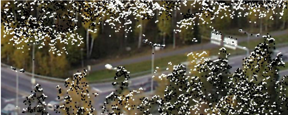
Figure 12. White spots are scanned from 800 m with a pulse repetition rate of 83 kHz (airborne TopoSys-1) and black points are scanned from 200 m at a rate of 7 kHz (helicopter-borne TopEye). (from Paper II)
