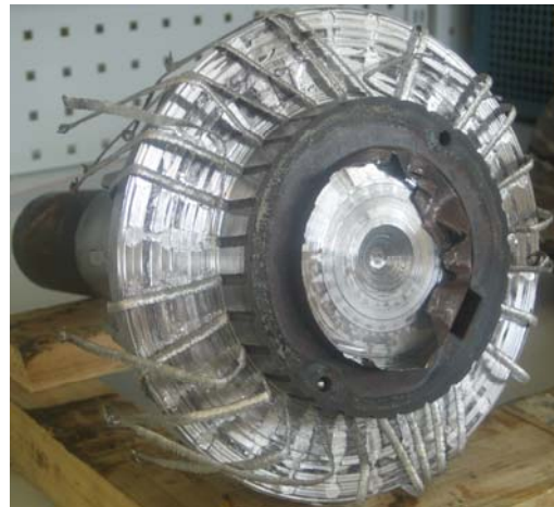
Figure 2.8 End of the rotor from which the sheets were machined.
