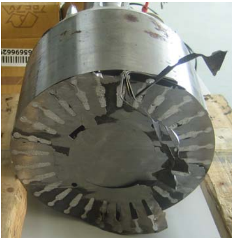
Figure 2.7 Half of the rotor of the cage-induction machine.
