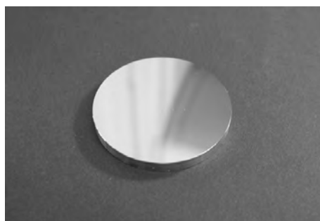
Figure 4.10: Diamond turned specimen for the laser fatigue experiments.
