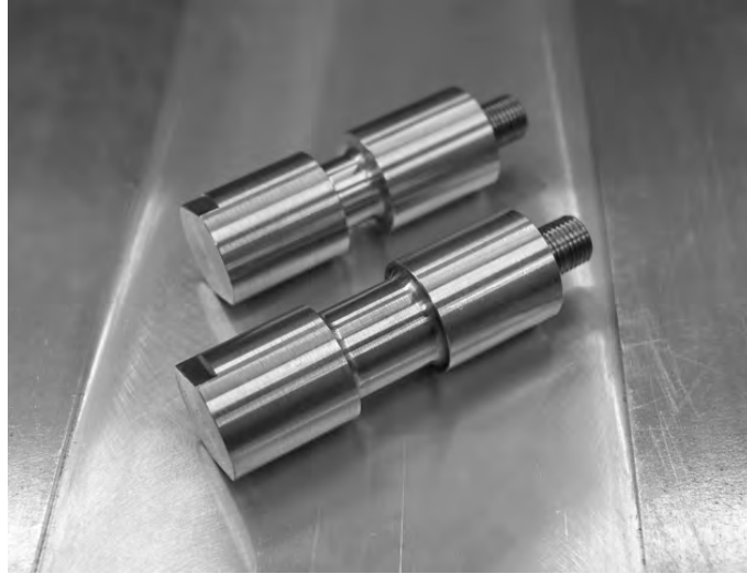
Figure 4.2: Diamond turned sonotrodes for ultrasonic fatigue experiments.
