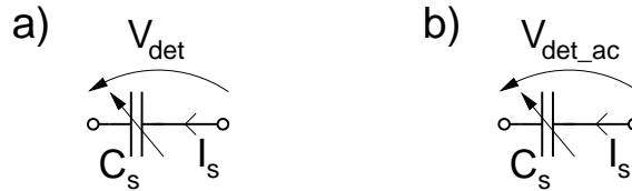
Figure 3.3: The use of (a) dc and (b) ac detection voltage for transforming the capacitive signal into charge/current.
