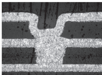
Figure 3.4: The cross-section image of two stacked vias, when the bottom via has been overfilled in the previous microvia fill step. The upper layer via has deformed due to the bump on top of the bottom layer via and the created interconnection is unreliable. [21]
