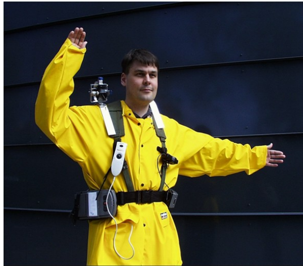
Figure 29. Command given by a gesture. Gesture is determined by detecting the yellow jacket and calculating the form of detection. User is also wearing a teleoperation device on his shoulders. This device can be used for direct teleoperation and for gesture recognition.
