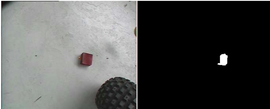
Figure 42. WorkPartner measuring the exact position of the litter. The original image and image thresholded with red.
