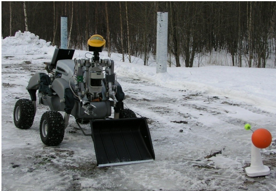
Figure 48. WorkPartner plowing snow. The white tubes behind the robot were used as beacons for the navigation system.
