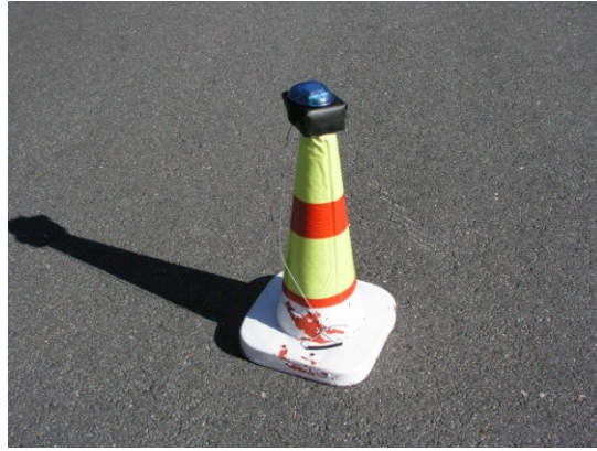
Figure 55. Active signs containing a GPS receiver, Bluetooth module, and a micro controller.
