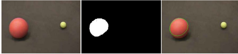
Figure 50. The original image, image thresholded with orange, and the orange circle that was found.
