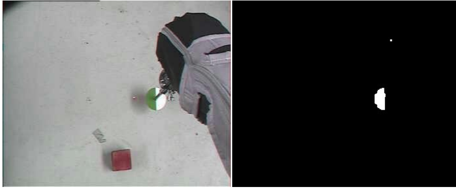
Figure 43. WorkPartner measuring the exact position of the gripper (or spike). The original image and image thresholded with green.
