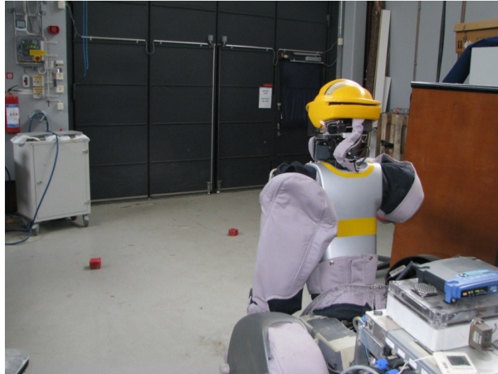
Figure 45. WorkPartner starts to pick up two pieces of litter. The litter items are red plastic foam cubes in front of the robot.
