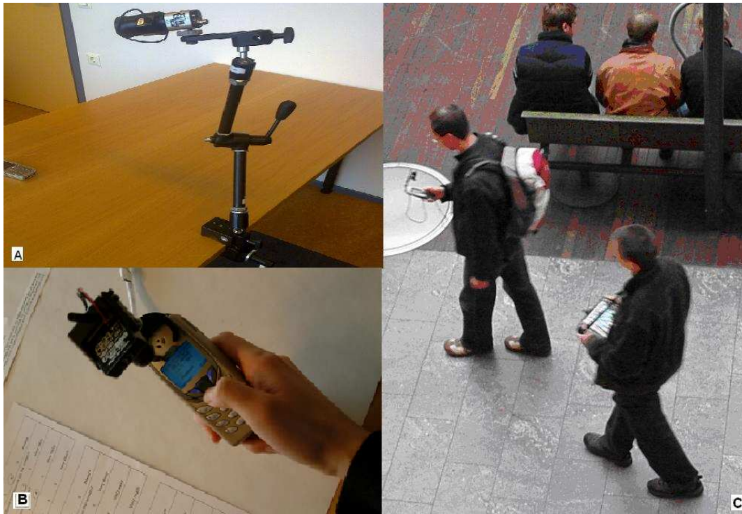
Figure 17 Evolution of test facilities in mobile service usability testing. First it was possible to use normal video camera in stand (17A), then minicamera was possible to use in laboratory (17B) and later in the field (17C).
