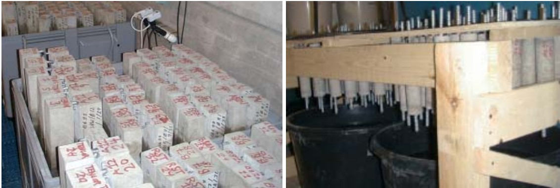
Fig. 32. Testing arrangements for beam (left) and cylinder (right) specimens.
