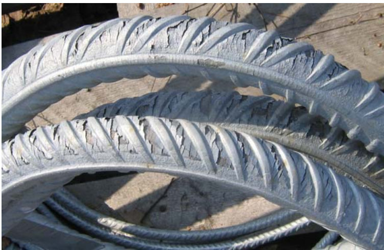
Fig. 14. Bent specimens after three years of storage outdoors 2 .
