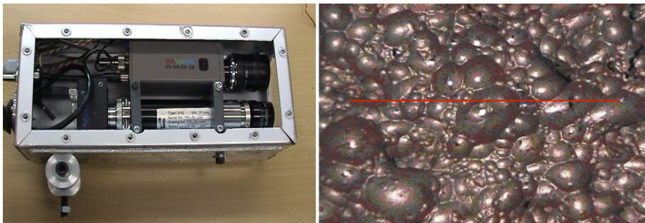
Fig. 6.1 RGB- and spectral data was obtained from same location simultaneously. The imaged line position is illustrated on the right (not in scale).
