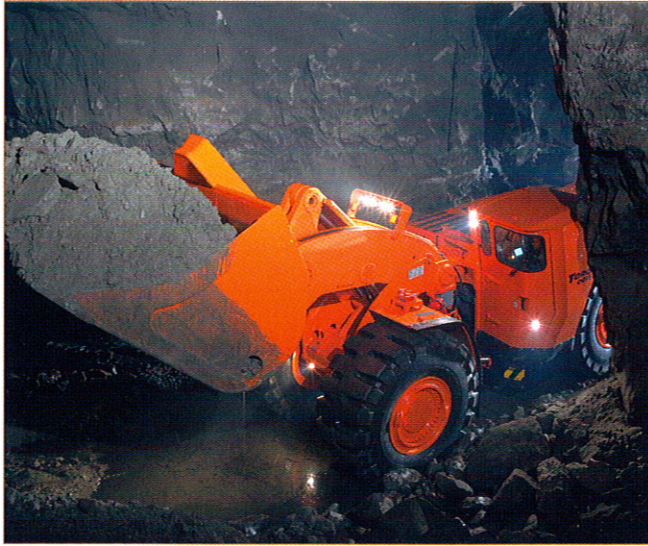
Fig. 3.5 A LHD loader with 21t capacity. (courtesy of Pyhäsalmi Mine Oy)
