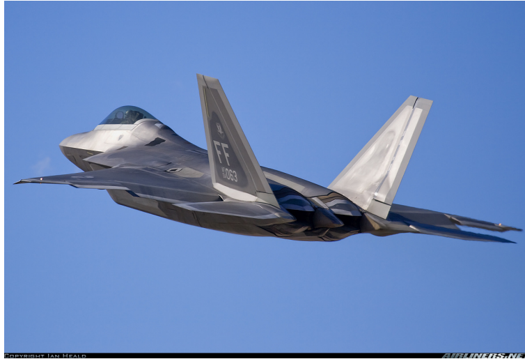
Figure 2.2: Lockheed-Martin/Boeing F-22 Raptor is a modern stealth fighter. Pay attention to the special shape of the aircraft and the hidden engine nozzles. Photo: Ian Heald.
